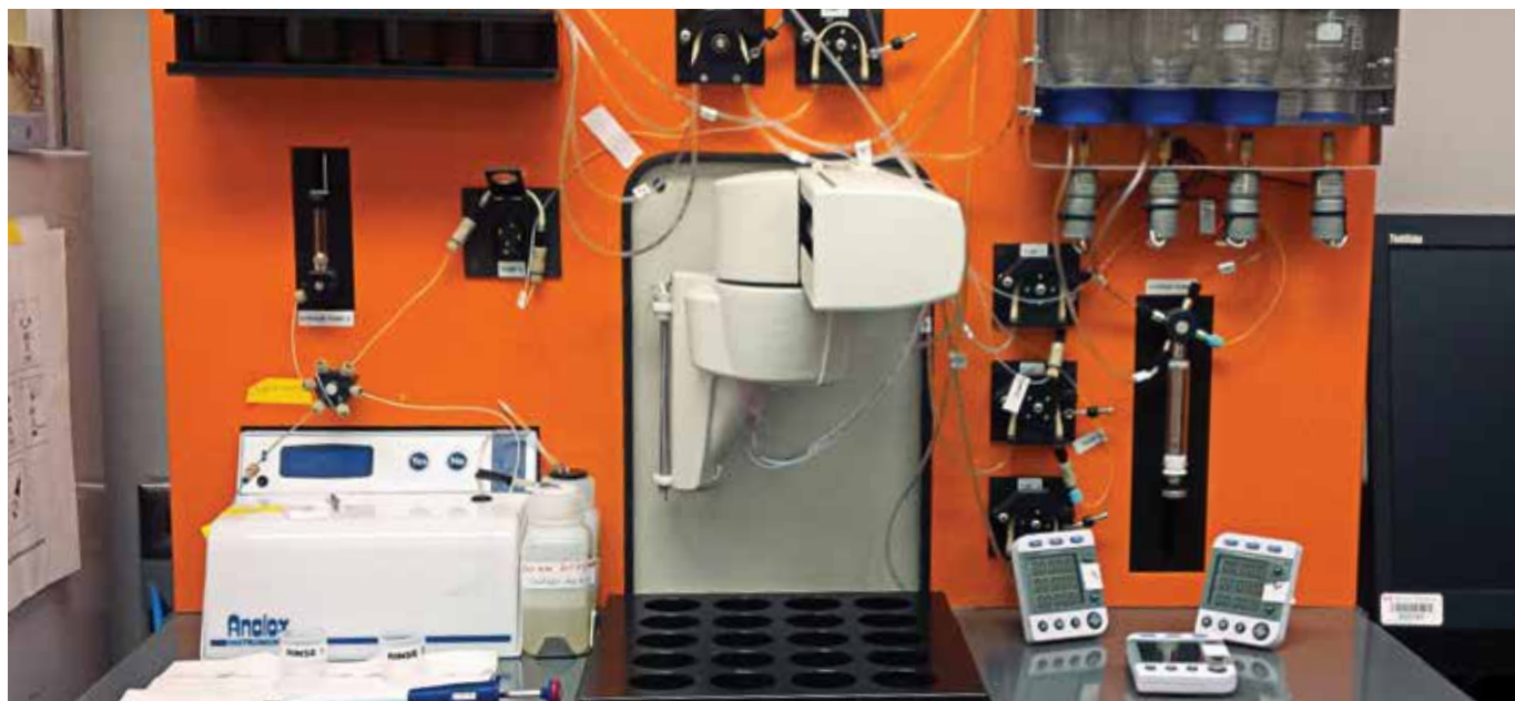
Prototype instrument purchased by Agriculture and Agri-Food Canada. This instrument simulates upper gut digestion of foods and measures the rate at which starch is digested in vitro and can be used to predict blood sugar responses when the same foods are eaten by human volunteers.
