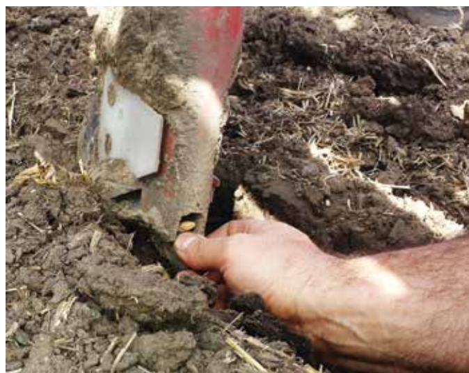
Rude's team found that soil openers posed problems for seeding faba bean. In this photo there is a jam at the opener exit.
