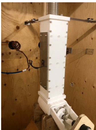
The vertical applicator (reactor) used in the RF process.
