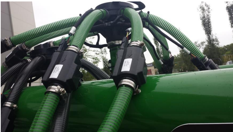
Figure 9. Straight-through blockage sensor.
