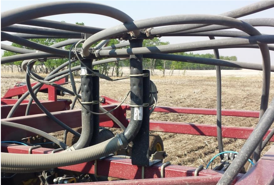
Figure 4. Tower type distribution manifold.
