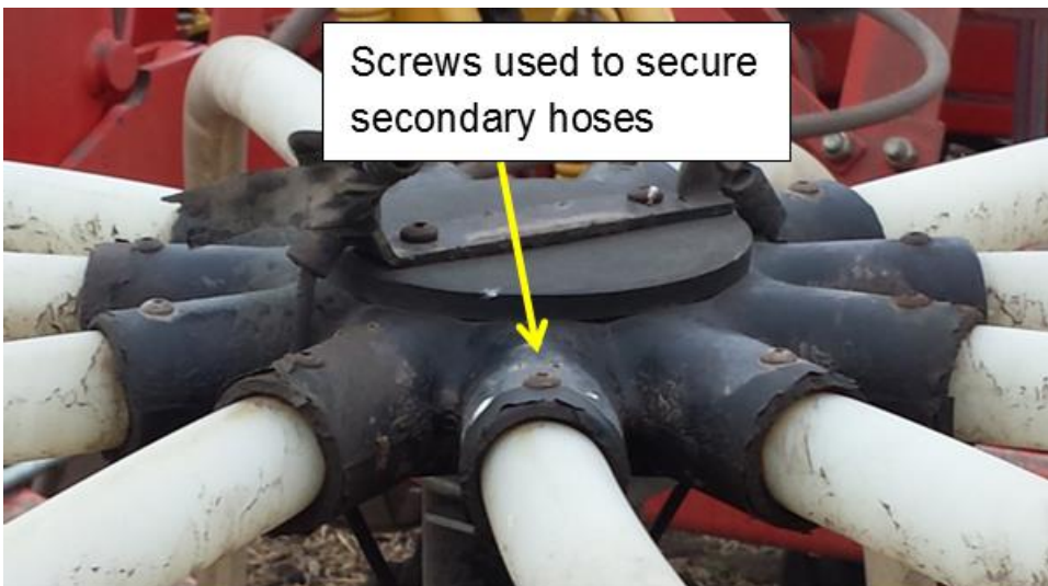
Figure 7. Screws used to secure secondary hoses to the distribution manifold.
