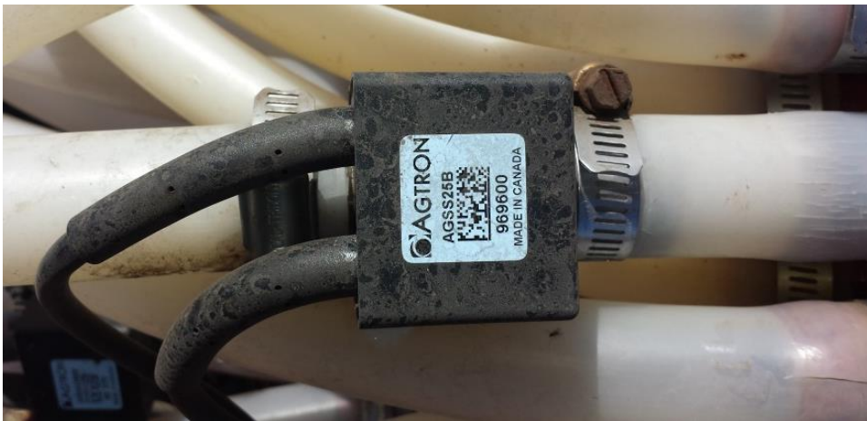
Figure 8. Straight-through blockage sensor.
