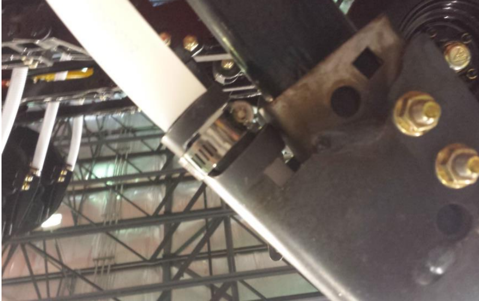
Figure 16. Updated Bourgault secondary hose clamp method.
