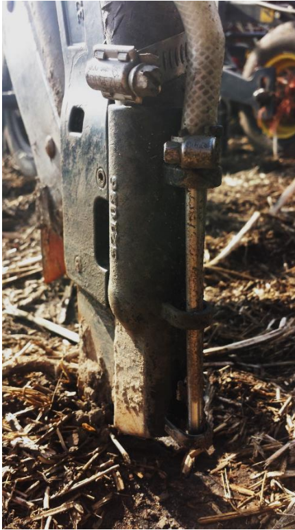
Figure 12. Narrow exit of seed tube.
