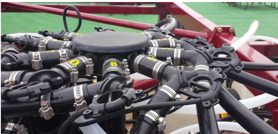
Figure 11. Blockage sensor with 90 degree path change.
