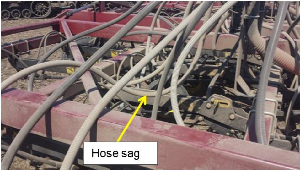
Figure 6. Sag in secondary hose caused a plug.
