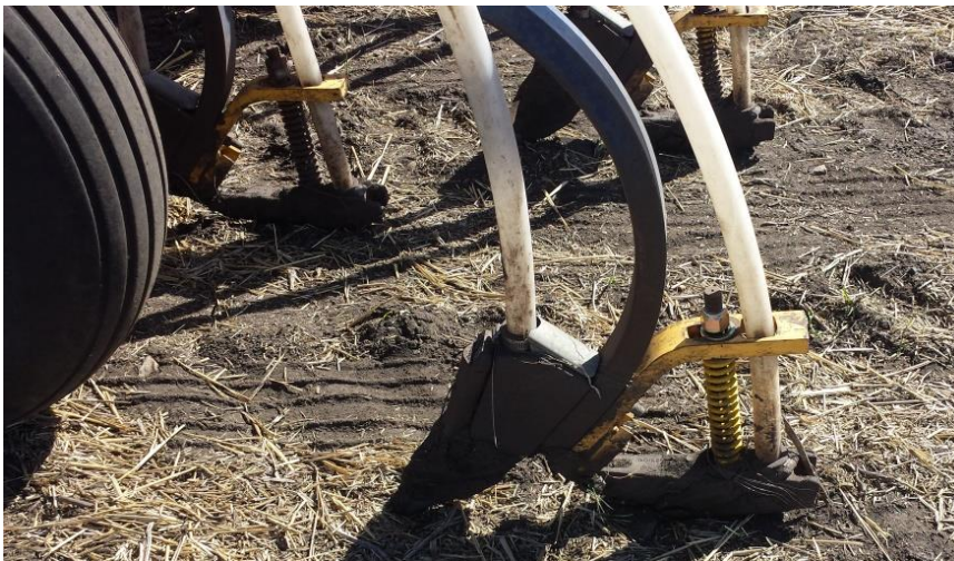
Figure 13. Straight through opener (rear hose applies seed).
