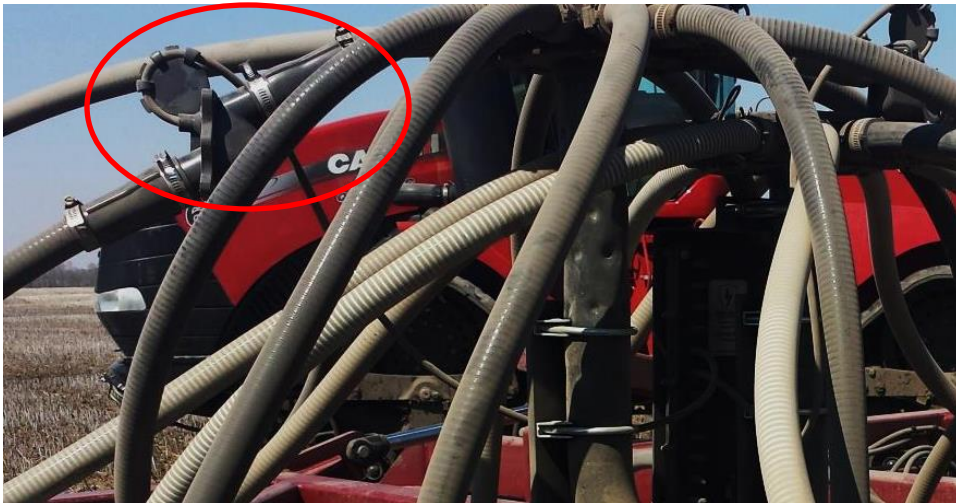
Figure 10. Blockage sensor with some flow path alteration.
