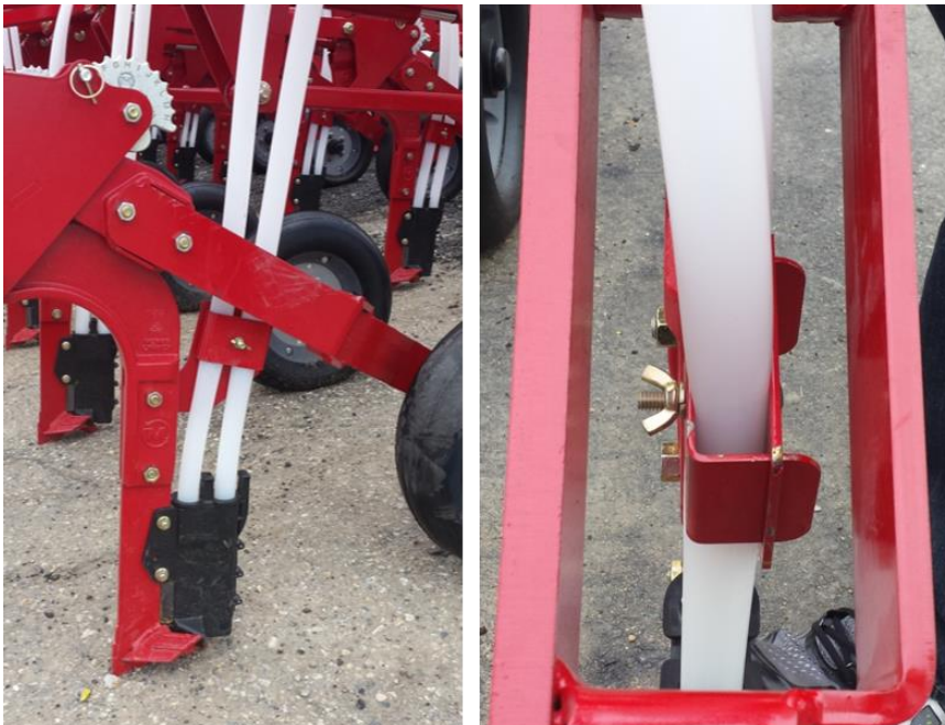
Figure 17. New Morris secondary hose retaining system.
